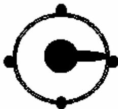
Normal 4 Cylinder Cap & Rotor
